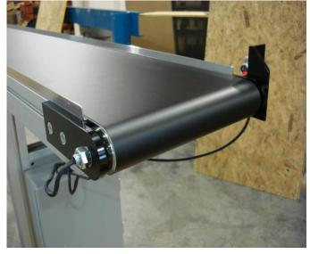
Drive Components Drive Roller- Control Card- 120 volt Power Supply
